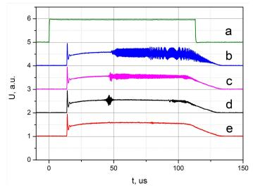
Figure 5. RF exciter trigger pulse (a) and output laser pulses measured with fast detector (b, c, d, e).
